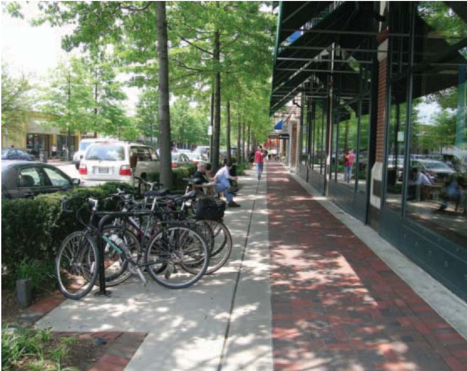
A safe and inviting sidewalk with shade trees and benches that serve as buffers from vehicular traffic
